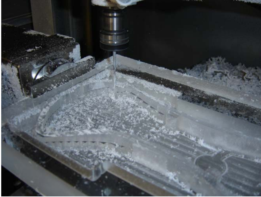
Figure 8.17 CNC Router Making Acrylic Piece
