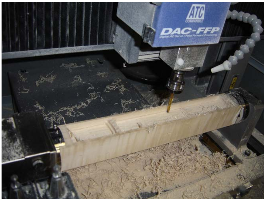
Figure 8.18 CNC Router Making Neck
