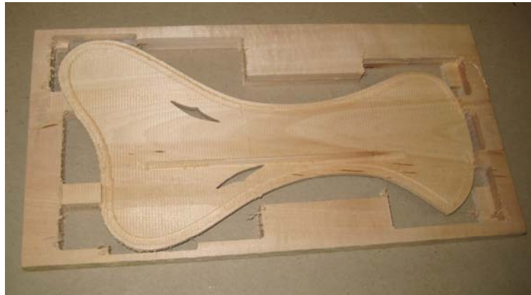
Figure 8.19 Wooden Top in Bounding Box from CNC Router
